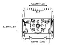
Make mounting holes on the wall according to the size shown in the picture. Use an electric drill to drill through the mounting holes on the lamp.
